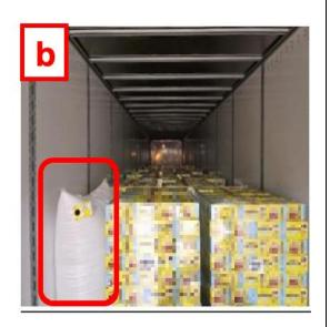
If air bagging a single pallet in the nose, center it & inflate airbags on either side.
