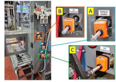
7. Use hand crank to adjust Hopper Bracket to numerical value required for new product:
